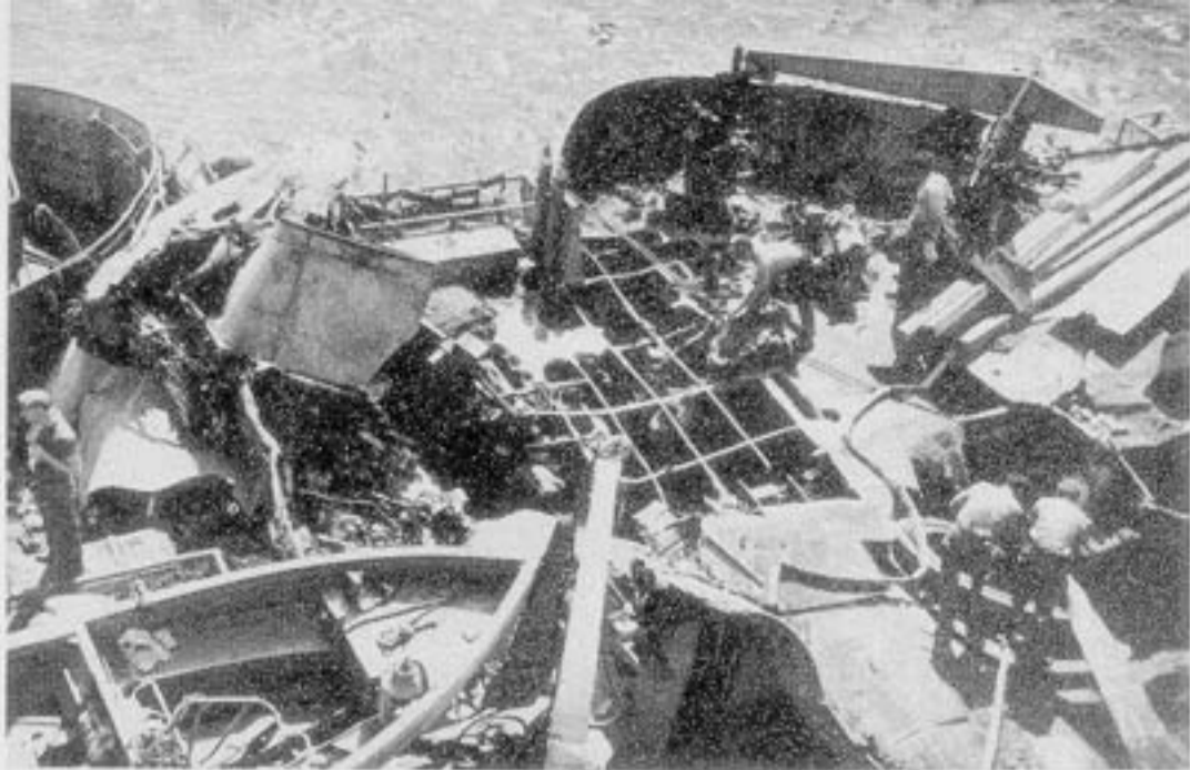
Photo 12-1: HUGH W. HADLEY (DD774). View of midship deckhouse, frames 130 to 150, in way of third Kamikaze crash and ensuing fire. Plane hit at base of director tower, left center, bomb at 40mm mount No.4, lower right.
