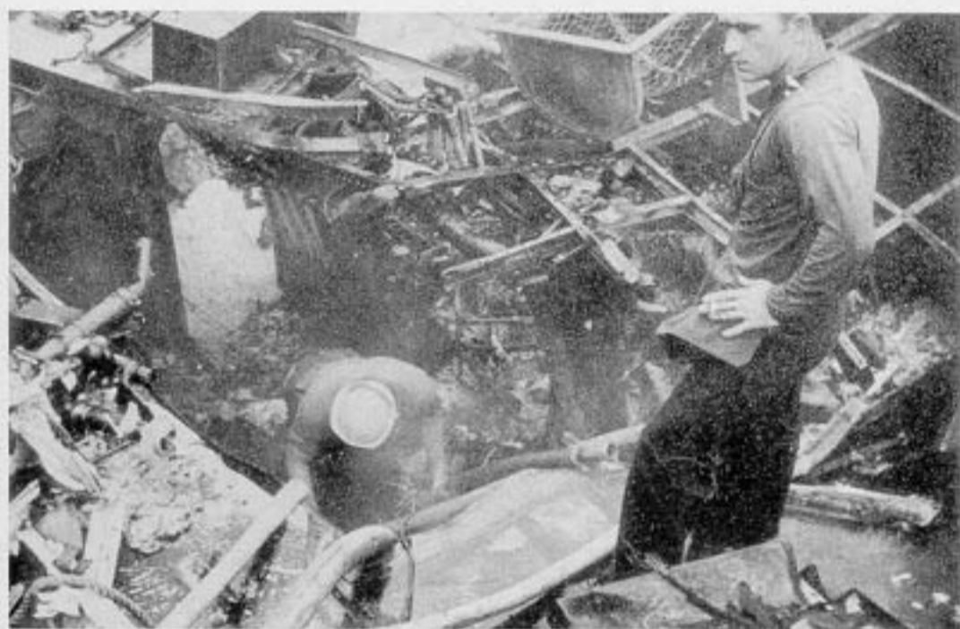
Photo 12-2: HUGH W. HADLEY (DD774). Close-up view of deckhouse top at frame 140 in way of plane crash and fire, looking down into officers' quarters aft.
