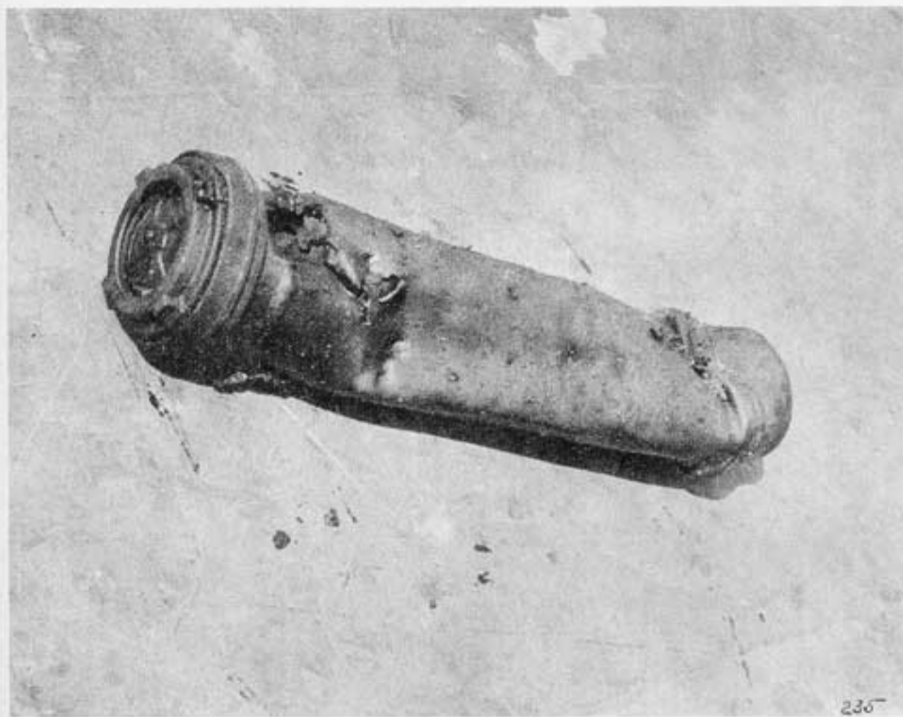
Photo 10-8: KILLEN (DD597). A typical burned-out powder cartridge can recovered from A-408-M. It has been crushed by blast, punctured by fragments, and powder inside burned out. Some unburned powder grains cling to the exterior surface.
