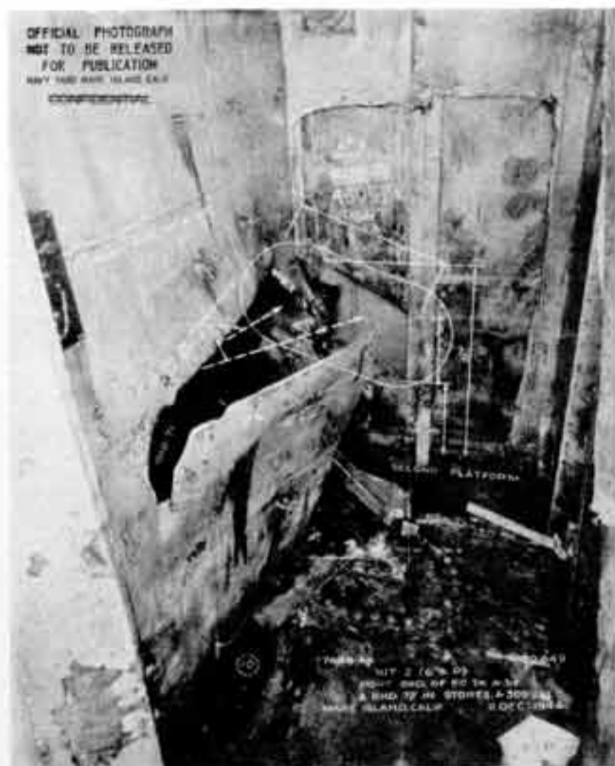
Photo 5-4: A.W. GRANT (DD649) - Hit #2. Hole in after port corner of A-3-F caused by 6-inch AP dud as it entered the forward fireroom. The projectile apparently broke into several large fragments before it emerged from A-3-F.
